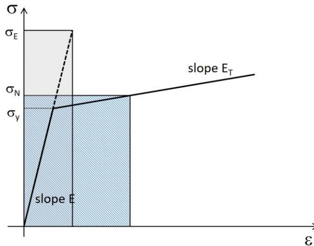
**Figure 6: Graphical representation of the Neuber correction**
