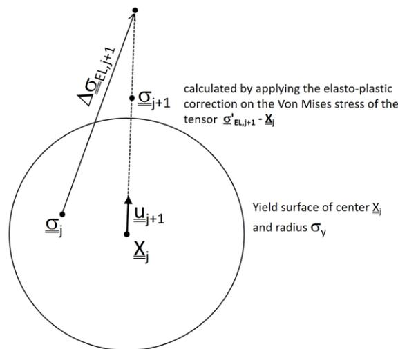
Figure 5: Elasto-plastic correction for a multiaxial cyclic stress
